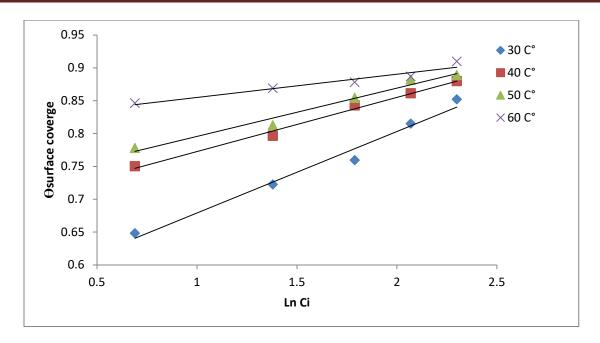
Figure (4.43): Temkin adsorption isotherm of Cordia myxa plant leaves (CML) extract inhibitor for aluminum corrosion in  $(1 \text{ M H}_3\text{PO}_4)$ .
