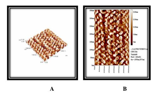
Figure (4.69): AFM images of aluminum surface immersed in (1M H<sub>3</sub>PO<sub>4</sub>).
