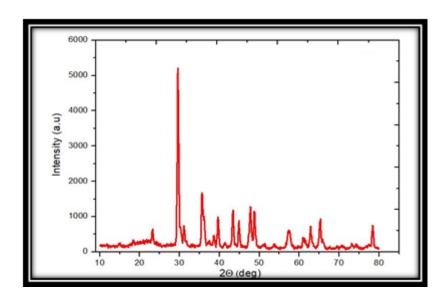
Figure (4.62): X-ray diffraction of aluminum surface.
