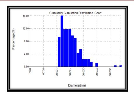
Figure (4.78): Granularity cumulating distribution and average diameter of aluminum alloy (AA6063-T5) surface immersed in (1M H<sub>3</sub>PO<sub>4</sub>).
