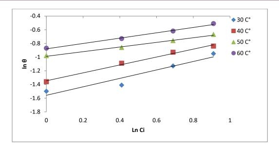
Figure (4.42): Freundlich adsorption isotherm of  $(TiO_2)$  nanomaterial for aluminum alloy (AA6063-T5) corrosion in  $(1MH_3PO_4 \text{ at pH of 4})$ .
