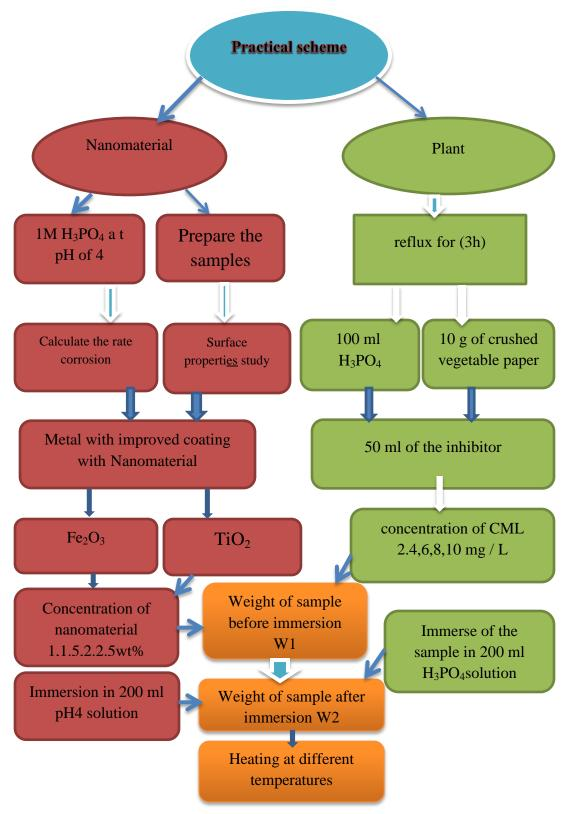
Figure (3.4): The experimental set up of corrosion study
