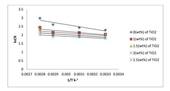
Figure (4.54): Arrhenius plot of aluminum alloy (AA6063 – T5) corrosion in  $(1MH_3PO_4 \text{ at pH of 4})$  containing various concentrations (TiO<sub>2</sub>) corrosion inhibitor at different temperatures.
