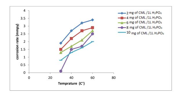
Figure (4.13): Effect of temperature on the corrosion rate of aluminum in  $(1 \text{ M H}_3 \text{PO}_4)$  at different inhibitor concentration (CML extract).
