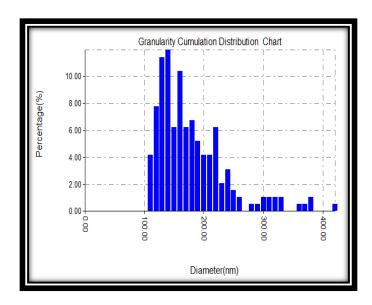
Figure (4.71): Granularity cumulating distribution of polished aluminum surface.
