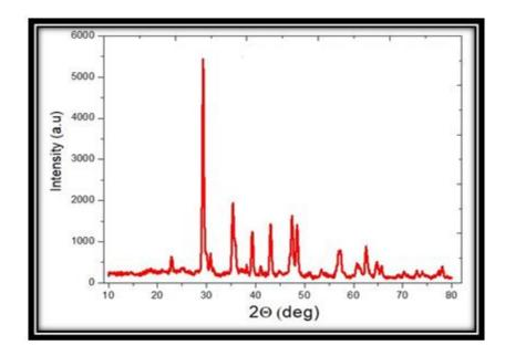
Figure (4.67) :X-ray diffraction of aluminum alloy (AA6063-T5) surface immersed in  $(1MH_3PO_4$  at pH of 4) in presence of  $(2.5wt\%TiO_2)$ .
