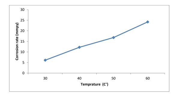
Figure (4.2): Effect of temperature on the corrosion rate of Cordia myxa leaves (CML) extract for aluminum alloy (AA6063 – T5) immersed in  $(1 \text{ M H}_3\text{PO}_4)$  for (3 h).
