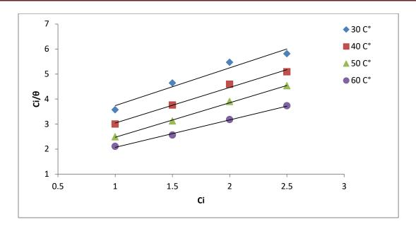
Figure (4.35): Langmuir adsorption isotherm of  $(TiO_2)$  nanomaterial for aluminum corrosion in  $(1MH_3PO_4 \text{ at pH of 4})$ .
