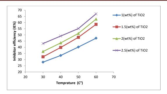
Figure (4.29): Effect of temperature on inhibition efficiency of (TiO<sub>2</sub>) nanomaterial for aluminum corrosion in (1MH<sub>3</sub>PO<sub>4</sub> at pH of 4).
