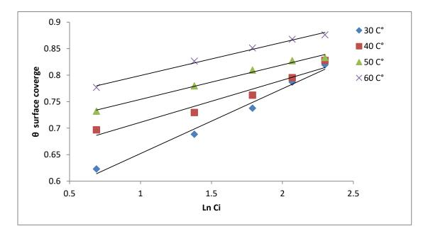
Figure (4.44): Temkin adsorption isotherm of Cordia myxa plant leaves(CML) extract inhibitor for aluminum alloy (AA6063-T5) corrosion in (1MH<sub>3</sub>PO<sub>4</sub>).
