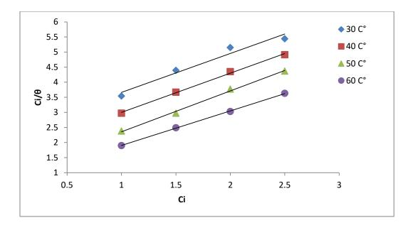
Figure (4.34): Langmuir adsorption isotherm of  $(Fe_2O_3)$  nanomaterial for aluminum alloy (AA6063-T5) corrosion in  $(1MH_3PO_4 \text{ at pH of 4})$ .
