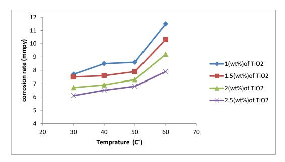
Figure (4.18): Effect of temperature on the corrosion rate of aluminum alloy (AA6063-T5) in(1M  $H_3PO_4$  at pH of 4) at different nanomaterial concentration (TiO<sub>2</sub>).
