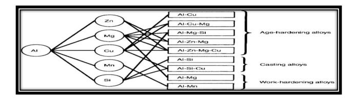
Figure (2.1) The principal aluminum alloys [50].
