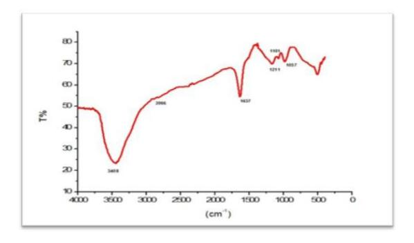
Figure (4.61.b):FTIR spectra of adsorbed film of CML extract on to aluminum surface after immersion (1M H<sub>3</sub>PO<sub>4</sub>).
