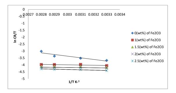
Figure (4.57): Transition state plot for aluminum corrosion in (1MH<sub>3</sub>PO<sub>4</sub> at pH of 4) in absence and presence of different concentrations of nanomaterial (Fe<sub>2</sub>O<sub>3</sub>) inhibitor.
