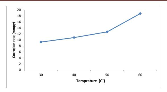
Figure (4.5): Effect of temperature on the corrosion rate of  $(TiO_2)$  nanomaterial for aluminum immersed in  $(1MH_3PO_4at\ pH\ of\ 4)$  for  $(3\ h)$ .
