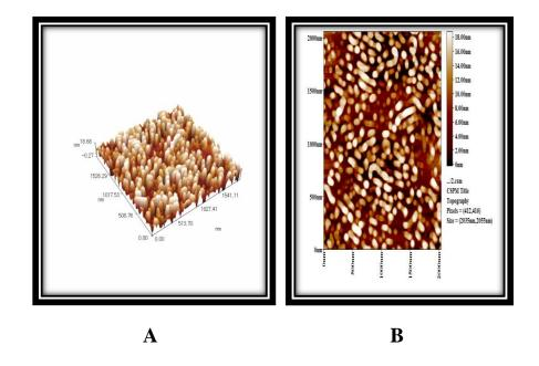
Figure (4.81): AFM images of aluminum surface immersed in (1M  $H_3PO_4$  at pH of 4) in presence of (2.5wt%Fe<sub>2</sub>O<sub>3</sub>) as nanomaterial inhibitor.
