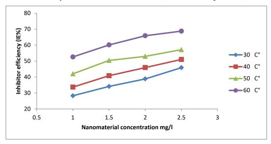
Figure (4.22): Effect of concentration of (Fe<sub>2</sub>O<sub>3</sub>) nanomaterial on inhibition efficiency of aluminum alloy (AA6063- T5) corrosion in (1MH<sub>3</sub>PO<sub>4</sub> at pH of 4).
