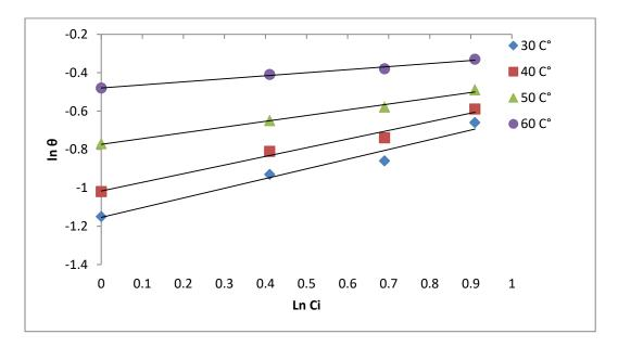
Figure (4.39): Freundlich adsorption isotherm of (Fe<sub>2</sub>O<sub>3</sub>) nanomaterial as corrosion inhibitor for aluminum corrosion in (1MH<sub>3</sub>PO<sub>4</sub> at pH of 4).
