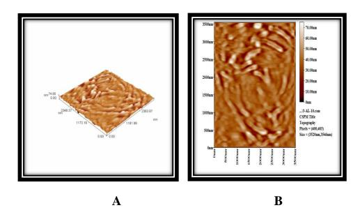
Figure (4.70) : AFM images of aluminum immersion in (1M  $H_3PO_4$ ) presence (10ml) of CML extract.
