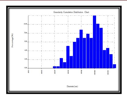
Figure (4.83): Granularity cumulating distribution and average diameter of aluminum surface immersed in (1M H<sub>3</sub>PO<sub>4</sub> at pH of 4).
