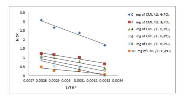
Figure (4.49): Arrhenius plot of aluminum corrosion in (1 MH<sub>3</sub>PO<sub>4</sub>) containing various concentrations Cordia myxa plant leaves (CML) extract as corrosion inhibitors.
