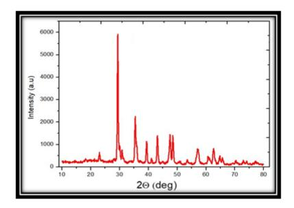
Figure (4.65) :X-ray diffraction of aluminum alloy (AA6063-T5) surface immersed in (1MH<sub>3</sub>PO<sub>4</sub> at pH of 4) in presence of (2.5wt%Fe<sub>2</sub>O<sub>3</sub>).
