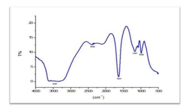
Figure (4.61.c):FTIR spectra of adsorbed film of CML extract on to aluminum alloy (AA6063-T5) surface after immersion (1M H<sub>3</sub>PO<sub>4</sub>).
