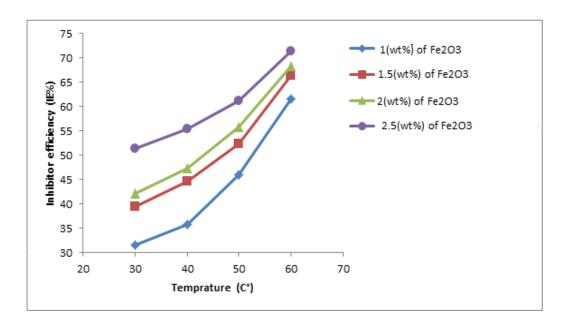
Figure (4.27): Effect of temperature on inhibition efficiency of  $(Fe_2O_3)$  nanomaterial for aluminum corrosion in  $(1M\ H_3PO_4\ at\ pH\ of\ 4)$ .
