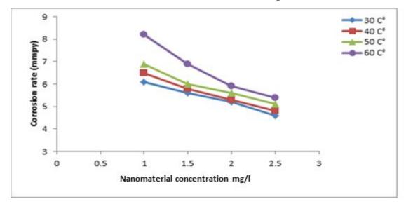
Figure (4.10):Effect of inhibitor concentrate on  $(Fe_2O_3)$  nanomaterial on the corrosion rate of aluminum alloy (AA6063- T5) immersed in in  $(1MH_3PO_4$  at pH of 4)for (3h).
