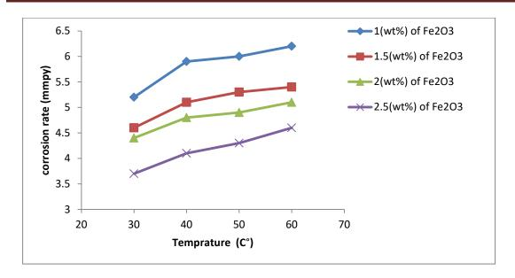
Figure (4.15): Effect of temperature on the corrosion rate of aluminum in  $(1MH_3PO_4 \text{ at pH of 4})$  at different nanomaterial concentration  $(Fe_2O_3)$ .
