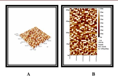
Figure (4.80 ): AFM images of aluminum surface immersed in (1M  $H_3PO_4$  at pH of 4).
