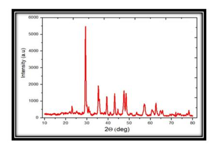
Figure (4.66) :X-ray diffraction of aluminum surface immersed in (1MH<sub>3</sub>PO<sub>4</sub> at pH of 4) in presence of (2.5wt%TiO<sub>2</sub>).
