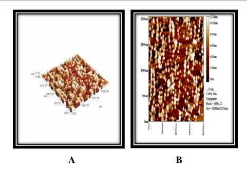
Figure (4.86): AFM images of aluminum alloy (AA6063-T5) surface immersed in  $(1MH_3PO_4$  at pH of 4).
