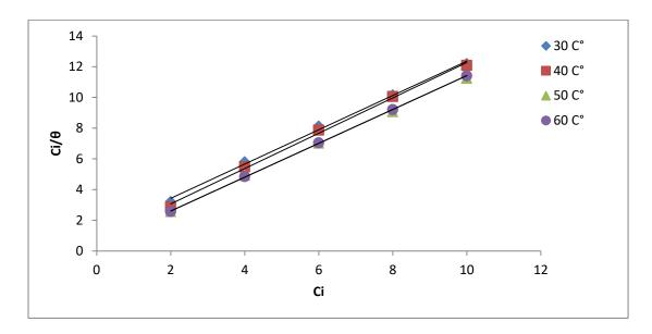
Figure (4.32): Langmuir adsorption isotherm of Cordia myxa plant leaves (CML) extract for aluminum alloy (AA6063-T5) corrosion in (1 M H<sub>3</sub>PO<sub>4</sub>).
