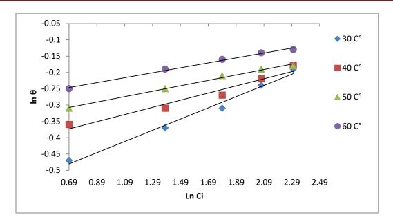
Figure (4.38): Freundlich adsorption isotherm of Cordia myxa plant leaves (CML) extract as corrosion inhibitor for aluminum alloy (AA6063-T5) corrosion in (1 M H<sub>3</sub>PO<sub>4</sub>).
