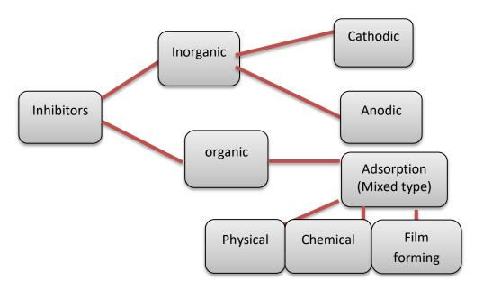
Figure (2.2): Shows classification of corrosion inhibitors .
