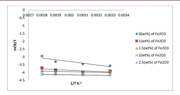
Figure (4.58): Transition state plot for aluminum alloy (AA6063-T5) corrosion in (1MH<sub>3</sub>PO<sub>4</sub> at pH of 4) in absence and presence of different concentrations of nanomaterial (Fe<sub>2</sub>O<sub>3</sub>) inhibitor.
