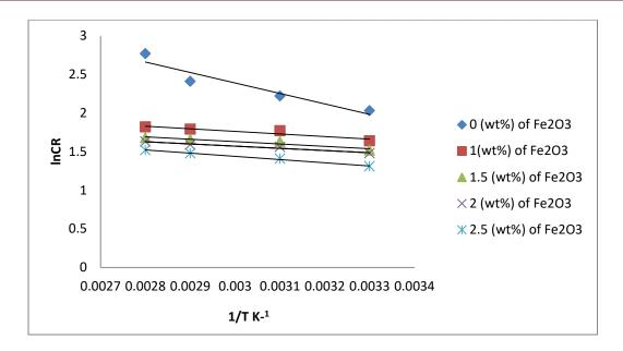
Figure (4.51): Arrhenius plot of aluminum corrosion in  $(1MH_3PO_4 \text{ at})$  pH of 4) containing various concentrations  $(Fe_2O_3)$  corrosion inhibitor at different temperatures .
