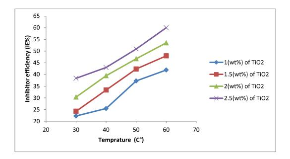
Figure (4.30): Effect of temperature on inhibition efficiency of  $(TiO_2)$  nanomaterial for aluminum alloy (AA6063- T5) corrosion in  $(1MH_3PO_4)$  at pH of 4).
