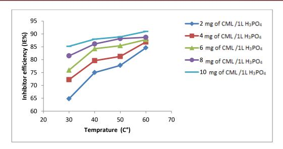
Figure (4.25): Effect of temperature on inhibitive efficiency of Cordia myxa plant leaves (CML) extract for aluminum corrosion in (1 M H<sub>3</sub>PO<sub>4</sub>).
