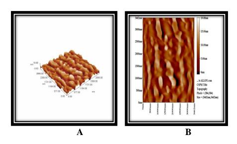
Figure (4.74): AFM images of polished aluminum alloy (AA6063-T5) surface.
