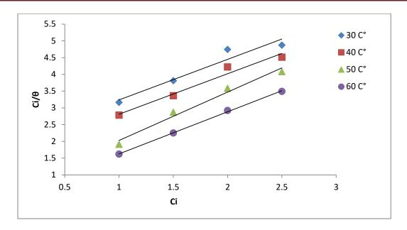
Figure (4.33): Langmuir adsorption isotherm of  $(Fe_2O_3)$  nanomaterial for aluminum corrosion in  $(1MH_3PO_4$  at pH of 4).
