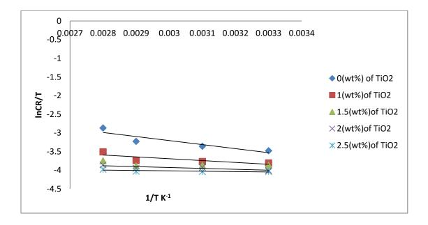
Figure (4.59): Transition state plot for aluminum corrosion in(1MH<sub>3</sub>PO<sub>4</sub> at pH of 4) in absence and presence of different concentrations of nanomaterial (TiO<sub>2</sub>) inhibitor.
