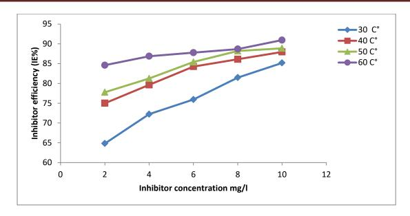
Figure (4.19): Effect of concentration of Cordia myxa plant leaves (CML) extract on inhibitive efficiency of aluminum corrosion in (1 M H<sub>3</sub>PO<sub>4</sub>).
