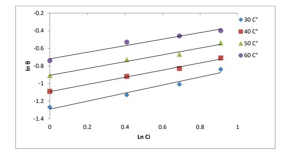
Figure(4.41): Freundlich adsorption isotherm of (TiO<sub>2</sub>) nanomaterial as corrosion inhibitor for aluminum corrosion in (1MH<sub>3</sub>PO<sub>4</sub> at pH of 4).
