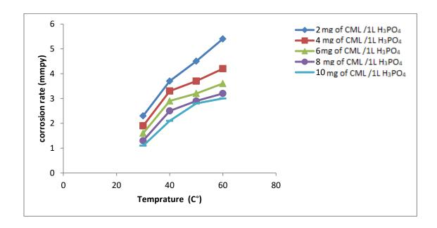
Figure (4.14): Effect of temperature on the corrosion rate of aluminum alloy (AA6063 - T5) in (1 M  $H_3PO_4$ ) at different inhibitor concentration (CML extract).
