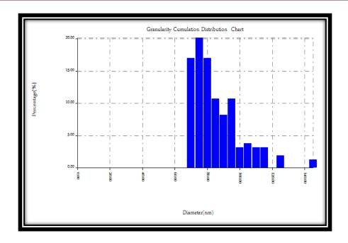
Figure (4.90): Granularity cumulating distribution and average diameter of aluminum alloy (AA6063-T5) surface immersed in (1MH<sub>3</sub>PO<sub>4</sub> at pH of 4) in presence of (2.5wt%Fe<sub>2</sub>O<sub>3</sub>).
