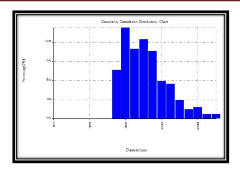
Figure (4.85): Granularity cumulating distribution and average diameter of aluminum surface immersed in  $(1MH_3PO_4 \text{ at pH of 4})$  in presence of  $(2.5\text{wt}\%\text{TiO}_2)$ .
