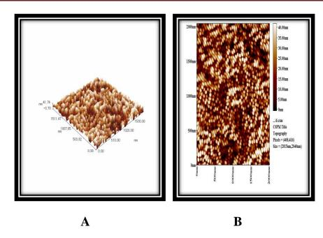
Figure (4.88): AFM images of aluminum alloy (AA6063-T5) surface immersed in (1MH<sub>3</sub>PO<sub>4</sub> at pH of 4) in presence of (2.5wt%TiO<sub>2</sub>) as nanomaterial inhibitor.
