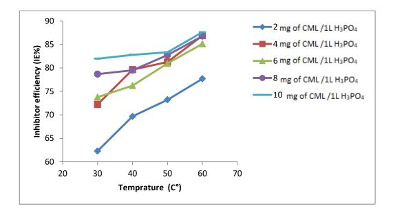
Figure (4.26): Effect of temperature on inhibition efficiency of Cordia myxa plant leaves (CML) extract for aluminum alloy (AA6063-T5) corrosion in (1 M  $H_3PO_4$ ).
