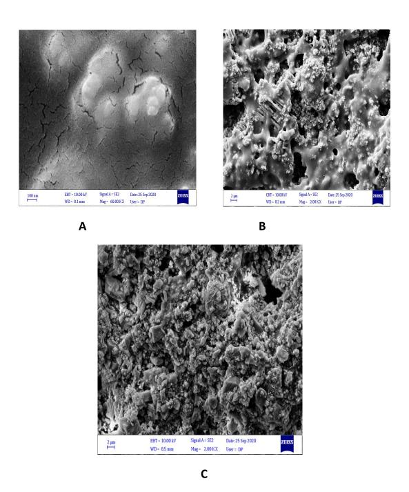
Figure (4.93): SEM images of aluminum alloy (AA6063-T5) surface corroded at (333 K) for (3 h): (A) aluminum alloy (AA6063-T5) surface only immersed in (1MH<sub>3</sub>PO<sub>4</sub> at pH of 4).(B) aluminum alloy (AA6063-T5) surface immersed in (1MH<sub>3</sub>PO<sub>4</sub> at pH of 4) in presence of (Fe<sub>2</sub>O<sub>3</sub>).(C) aluminum alloy (AA6063-T5) surface immersed in (1MH<sub>3</sub>PO<sub>4</sub> at pH of 4) in Presence of (TiO<sub>2</sub>).
