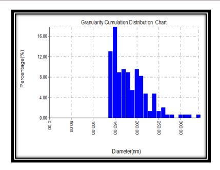
Figure (4.77): Granularity cumulating distribution and average diameter of polished aluminum alloy (AA6063-T5) surface.
