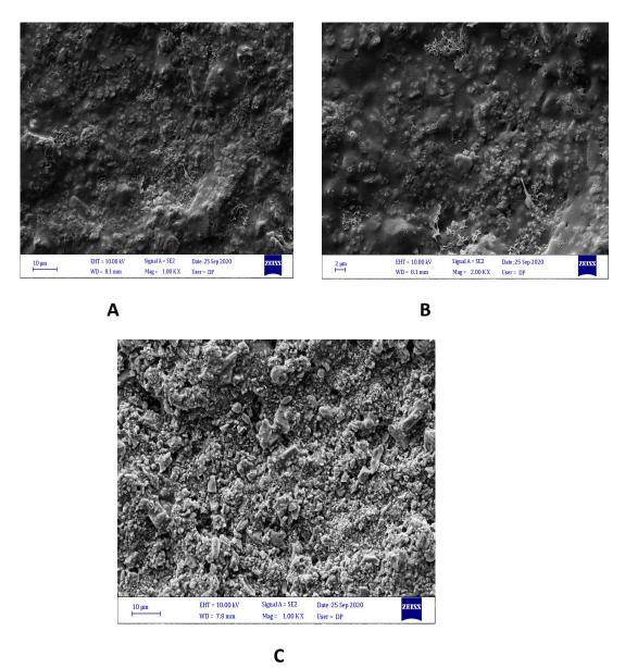
Figure (4.92): SEM images of aluminum surface corroded at (333 K) for (3 h): (A) aluminum surface only immersed in (1MH<sub>3</sub>PO<sub>4</sub> at pH of 4).(B) aluminum surface immersed in (1MH<sub>3</sub>PO<sub>4</sub> at pH of 4) in presence of (Fe<sub>2</sub>O<sub>3</sub>).(C) aluminum surface immersed in (1MH<sub>3</sub>PO<sub>4</sub> at pH of 4) in presence of (TiO<sub>2</sub>).
