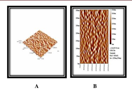
Figure (4.76) : AFM images of aluminum alloy (AA6063-T5) immersed in  $(1MH_3PO_4)$  in presence of (10ml) of CML extract.
