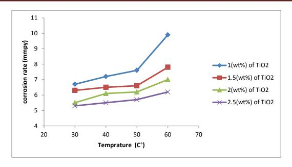
Figure (4.17): Effect of temperature on the corrosion rate of aluminum in  $(1MH_3PO_4at\ pH\ of\ 4)$  at different nanomaterial concentration  $(TiO_2)$ .
