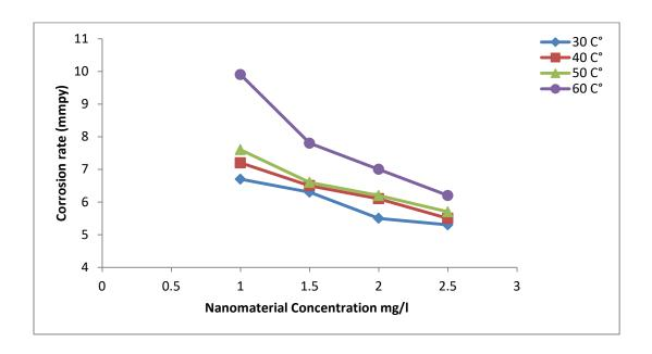
Figure (4.11): Effect of inhibitor concentration (TiO<sub>2</sub>) nanomaterial on the corrosion rate of aluminum immersed in (1MH<sub>3</sub>PO<sub>4</sub> at pH of 4) for (3h).
