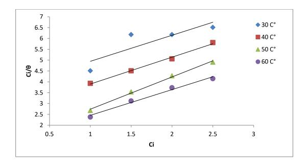
Figure (4.36): Langmuir adsorption isotherm of  $(TiO_2)$  nanomaterial for aluminum alloy (AA6063-T5) corrosion in  $(1MH_3PO_4 \text{ at pH of 4})$ .
