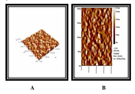
Figure (4.87): AFM images of aluminum alloy (AA6063-T5) surface immersed in  $(1M H_3PO_4 \text{ at pH of 4})$  in presence of  $(2.5\text{wt}\% Fe_2O_3)$  as nanomaterial inhibitor.
