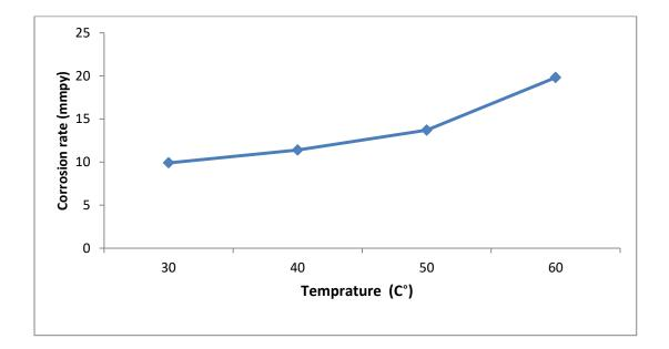
Figure (4.6): Effect of temperature on the corrosion rate of (TiO<sub>2</sub>) nanomaterial for aluminum alloy (AA6063- T5) immersed in (1MH<sub>3</sub>PO<sub>4</sub> at pH of 4) for (3 h).
