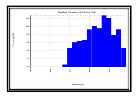
Figure (4.89): Granularity cumulating distribution and average diameter of aluminum alloy (AA6063-T5) surface immersed in (1MH<sub>3</sub>PO<sub>4</sub> at pH of 4).
