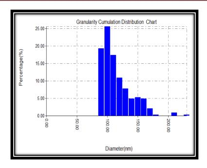
Figure (4.79): Granularity cumulating distribution and average diameter of aluminum alloy (AA6063-T5) immersed in (1MH<sub>3</sub>PO<sub>4</sub>) in presence of (10ml) of CML extract.
