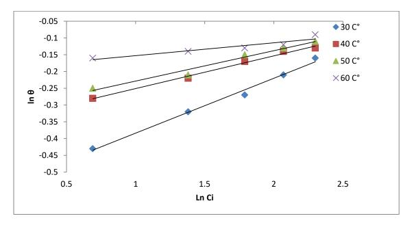
Figure (4.37): Freundlich adsorption isotherm of Cordia myxa plant leaves (CML) extract as corrosion inhibitor for aluminum corrosion in (1 M H<sub>3</sub>PO<sub>4</sub>).
