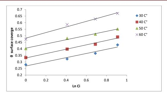
Figure (4.47): Temkin adsorption isotherm of nanomaterial ( $TiO_2$ ) inhibitor for aluminum corrosion in ( $1M H_3PO_4$  at pH of 4).
