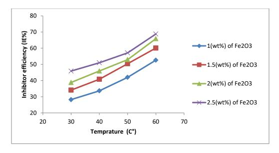
Figure (4.28): Effect of temperature on inhibition efficiency of  $(Fe_2O_3)$  nanomaterial for aluminum alloy(AA6063-T5) corrosion in  $(1MH_3PO_4)$  at pH of 4).
