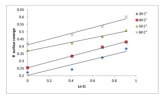
Figure (4.48): Temkin adsorption isotherm of nanomaterial ( $TiO_2$ ) inhibitor for aluminum alloy (AA6063-T5) corrosion in (1M  $H_3PO_4$  at pH of 4).
