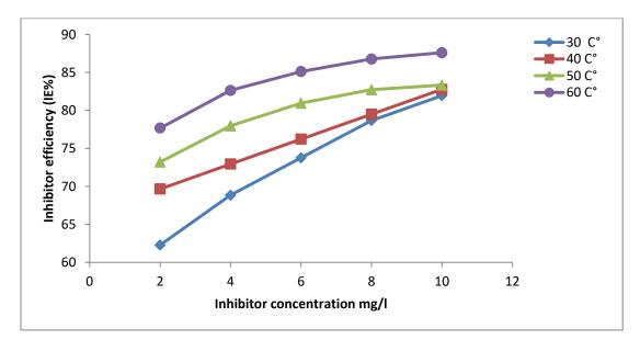
Figure (4.20): Effect of concentration of Cordia myxa plant leaves (CML) extract on inhibition efficiency of aluminum alloy (AA6063-T5) corrosion in (1 M H<sub>3</sub>PO<sub>4</sub>).
