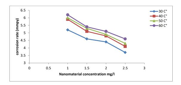
Figure (4.9): Effect of inhibitor concentration on  $(Fe_2O_3)$  nanomaterial on the corrosion rate of aluminum immersed in  $(1MH_3PO_4 \text{ at pH of 4})$  for (3 h).
