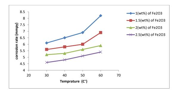
Figure (4.16): Effect of temperature on the corrosion rate of aluminum alloy in  $(1MH_3PO_4 \text{ at pH of 4})$  at different nanomaterial concentration  $(Fe_2O_3)$ .
