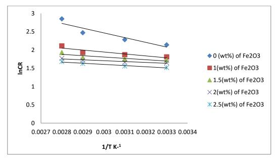
Figure (4.52): Arrhenius plot of aluminum alloy (AA6063 - T5) corrosion in (1MH<sub>3</sub>PO<sub>4</sub> at pH of 4) containing various concentrations (Fe<sub>2</sub>O<sub>3</sub>) corrosion inhibitor at different temperatures.
