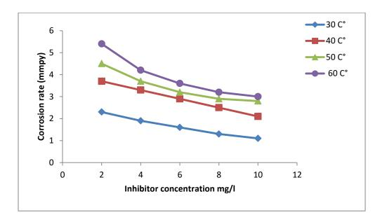
Figure (4.8): Effect of inhibitor concentration (CML extract) on the corrosion rate of aluminum alloy (AA6063 - T5) immersed in (1 M  $H_3PO_4$ ) for (3 h).
