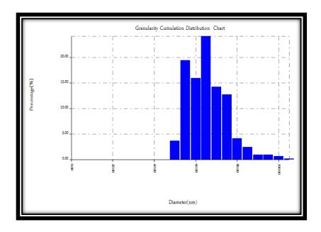
Figure (4.91): Granularity cumulating distribution and average diameter of aluminum alloy (AA6063-T5) surface immersed in (1MH<sub>3</sub>PO<sub>4</sub> at pH of 4) in presence of (2.5wt%TiO<sub>2</sub>).
