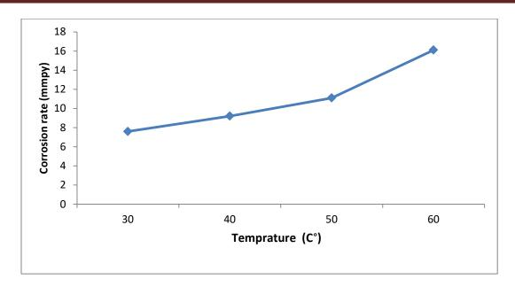
Figure (4.3): Effect of temperature on the corrosion rate of  $(Fe_2O_3)$  nanomaterial for aluminum immersed in  $(1MH_3PO_4$  at pH of 4) for (3 h).
