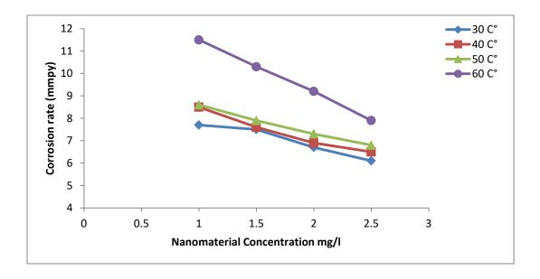
Figure (4.12): Effect of inhibitor concentration ( $TiO_2$ ) nanomaterial on the corrosion rate of aluminum alloy(AA6063-T5) immersed in ( $1MH_3PO_4$  at pH of 4) for (3h).
