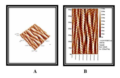
Figure (4.75 ): AFM images of aluminum alloy (AA6063-T5) surface immersed in  $(1M\ H_3PO_4)$ .
