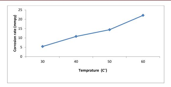
Figure (4.1): Effect of temperature on the corrosion rate of Cordia myxa leaves(CML) extract for aluminum immersed in  $(1 \text{ M H}_3 \text{ PO}_4)$  for (3 h).
