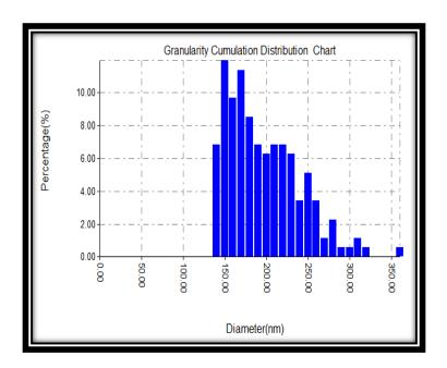
Figure (4.73): Granularity cumulating distribution and average diameter of aluminum immersed in  $(1M\ H_3PO_4)$  presence of (10ml) of CML extract.
