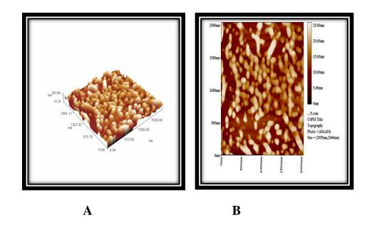
Figure (4.82): AFM images of aluminum surface immersed in (1M  $H_3PO_4$  at pH of 4) in presence of (2.5wt%TiO<sub>2</sub>) as nanomaterial inhibitor.
