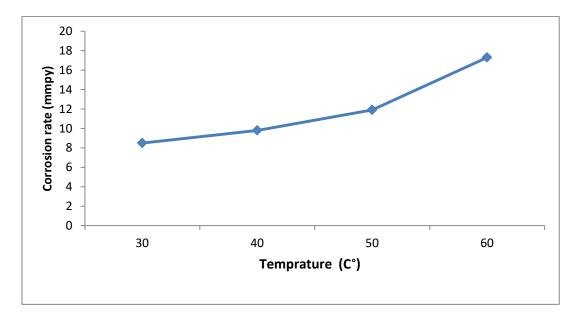
Figure (4.4): Effect of temperature on the corrosion rate of (Fe<sub>2</sub>O<sub>3</sub>) nanomaterial for aluminum alloy (AA6063- T5) immersed in (1MH<sub>3</sub>PO<sub>4</sub> at pH of 4) for (3 h).
