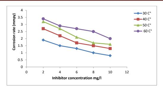
Figure (4.7): Effect of inhibitor concentration (CML extract) on the corrosion rate of aluminum immersed in  $(1 \text{ M H}_3\text{PO}_4)$  for (3 h).
