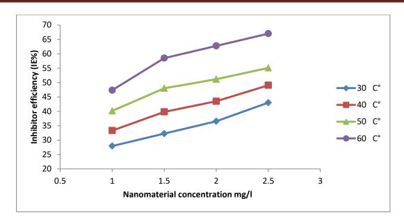
Figure (4.23): Effect of concentration of  $(TiO_2)$  nanomaterial on inhibition efficiency of aluminum corrosion in  $(1MH_3PO_4 \text{ at pH of 4})$ .
