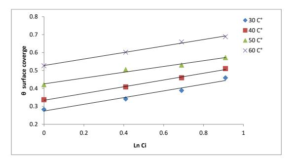
Figure (4.46): Temkin adsorption isotherm of nanomaterial ( $Fe_2O_3$ ) for aluminum alloy (AA6063 T5) corrosion in (1M  $H_3PO_4$  at pH of 4).
