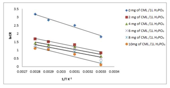
Figure (4.50):Arrhenius plot of aluminum alloy (AA6063 – T5) corrosion in (1 M H<sub>3</sub>PO<sub>4</sub>) containing various concentrations Cordia myxa plant leaves (CML) extract at different temperatures as corrosion inhibitors.
