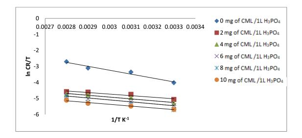
Figure (4.55): Transition state plot for aluminum corrosion in  $(1 \text{ M H}_3 \text{PO}_4)$  in absence and presence of different concentrations of (CML) extract.
