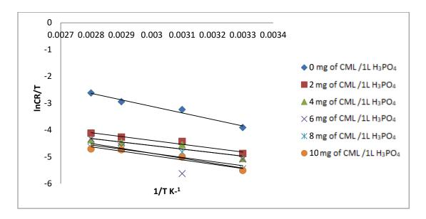
Figure (4.56): Transition state plot for aluminum alloy (AA6063 - T5) corrosion in (1 M  $_3$ PO $_4$ ) in absence and presence of different concentrations of (CML) extract.
