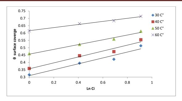
Figure (4.45): Temkin adsorption isotherm of nanomaterial ( $Fe_2O_3$ ) inhibitor for aluminum corrosion in (1M  $H_3PO_4$  at pH of 4).
