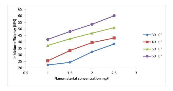
Figure (4.24): Effect of concentration of (TiO<sub>2</sub>) nanomaterial on inhibition efficiency of aluminum alloy (AA6063-T5) corrosion in (1MH<sub>3</sub>PO<sub>4</sub> at pH of 4).
