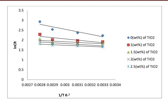
Figure (4.53): Arrhenius plot of aluminum corrosion in  $(1MH_3PO_4 \text{ at pH of 4})$  containing various concentrations  $(TiO_2)$  corrosion inhibitor at different temperatures.
