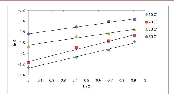
Figure (4.40): Freundlich adsorption isotherm of  $(Fe_2O_3)$  nanomaterial as corrosion inhibitor for aluminum alloy (AA6063-T5) corrosion in  $(1MH_3PO_4)$  at pH of 4).
