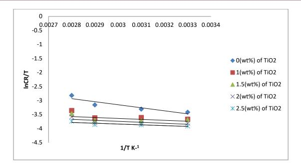
Figure (4.60): Transition state plot for aluminum alloy (AA6063-T5) corrosion in(1MH<sub>3</sub>PO<sub>4</sub> at pH of 4) in absence and presence of different concentrations of nanomaterial (TiO<sub>2</sub>) inhibitor.
