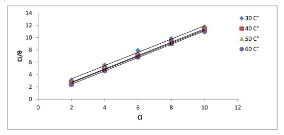
Figure (4.31): Langmuir adsorption isotherm of Cordia myxa plant leaves (CML) extract for aluminum corrosion in  $(1 \text{ M H}_3\text{PO}_4)$ .
