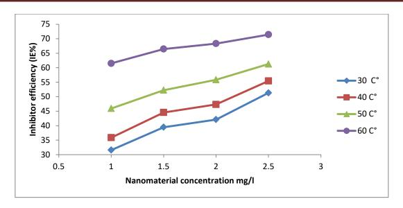
Figure (4.21): Effect of concentration of (Fe<sub>2</sub>O<sub>3</sub>) nanomaterial on inhibition efficiency of aluminum corrosion in (1MH<sub>3</sub>PO<sub>4</sub> at pH of 4).
