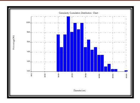
Figure (4.84): Granularity cumulating distribution and average diameter of aluminum surface immersed in  $(1MH_3PO_4 \text{ at pH of 4})$  in presence of  $(2.5\text{wt}\%\text{Fe}_2\text{O}_3)$ .
